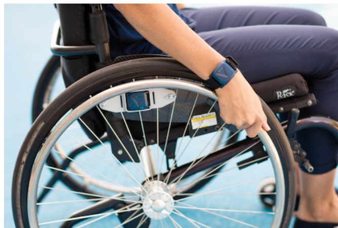
Figure D.3 – Sensor placement of the wheeling detection algorithm (created by Rehabilitation Engineering Laboratory, ETH Zurich).
