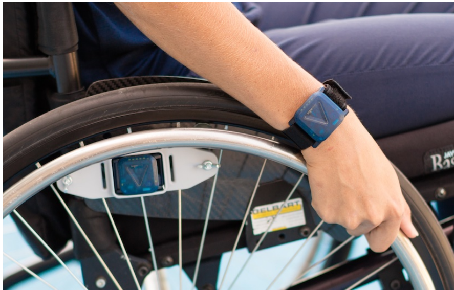
Figure 1.1 – Exemplary illustration of a wrist-worn ZurichMOVE sensor module and a second sensor module attached to the spokes of the wheel (created by Rehabilitation Engineering Laboratory, ETH Zurich).
