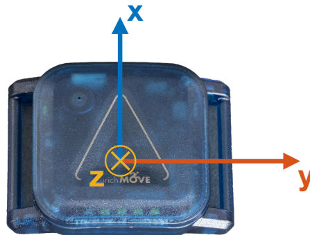
Figure D.1 – The ZurichMOVE sensor and its coordinate system (created by Rehabilitation Engineering Laboratory, ETH Zurich).
