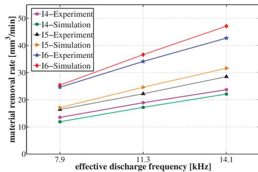
Fig. 8. MRR obtained for a brass workpiece
