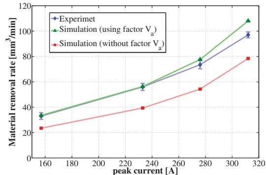
Fig. 9. MRR obtained for a diamond grinding wheel
