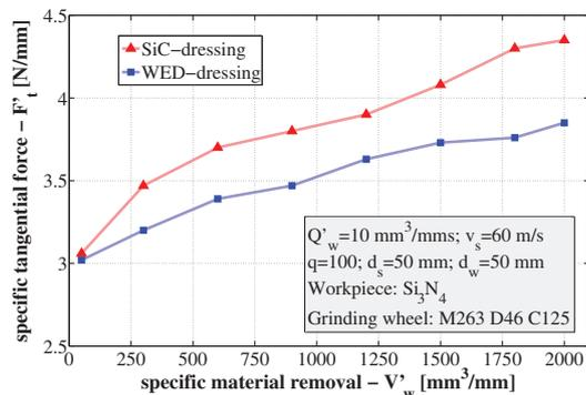
Fig. 3. Grinding forces in WED-dressing and SiC-dressing
