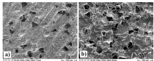
Fig. 2. SEM-micrographs a) SiC-dressed and b) WED-dressed wheels
