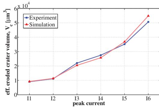
Fig. 7. Effective volume of eroded material  $V_c$
