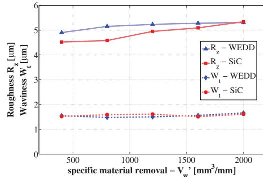
Fig. 4. Workpiece surface quality (SiC-dressing vs. WEDD)
