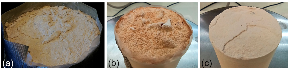
Fig. 6 a Decay and efflorescences in Migné specimens contaminated with 1 wt% \text{Na}_2\text{SO}_4 at the end of the test, before brushing off the evaporation surface; b decay in Migné specimen contaminated with 5 wt% \text{Na}_2\text{SO}_4 at the end of the
