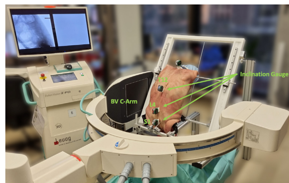
Fig. 1. Experiment setup with image intensifier, stabilizing frame and the inclination gauges in place.
