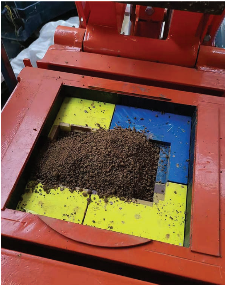
9 The earth material is loaded into the 3D-printed mold before closing the lid of the press
