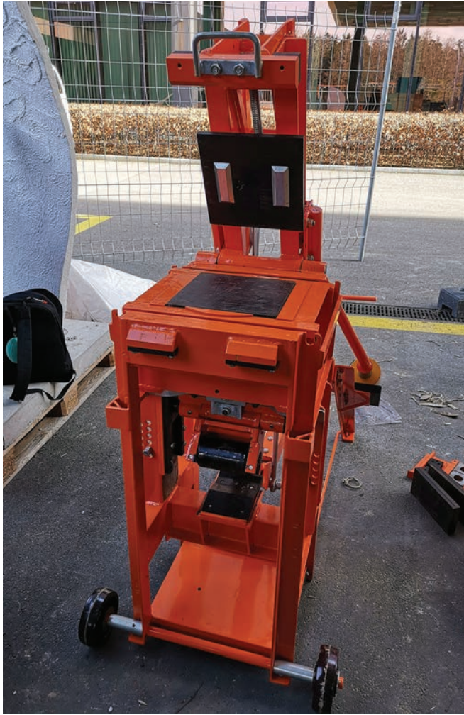
7 The compressed earth block (CEB) press with the default steel mold
