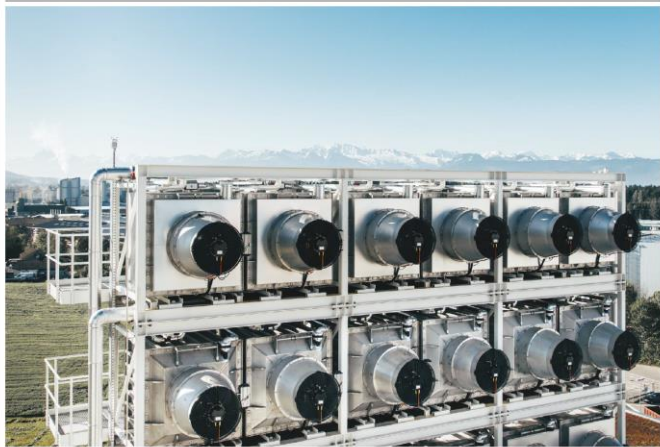
Climevents' plant for direct air capture in Iceland removes carbon dioxide permanently from the atmosphere.
