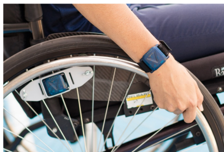
Figure 4.1: Participant wearing sensor modules attached to the right wrist and the wheelchair wheel.
