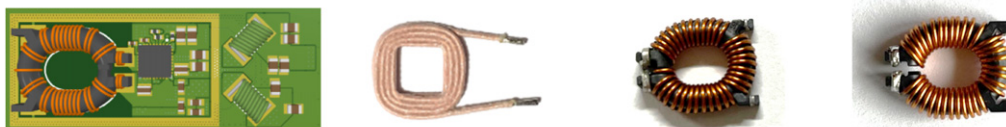
Figure 5. From the left hand side: a picture of a complete design of a DC-DC converter block; a photo of a Litz wire solenoid; a photo of a toroidal inductor supplied by the first supplier; a photo of a toroidal inductor supplied by the second supplier.
