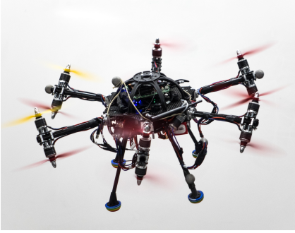
Figure 6.2: The omnidirectional flying vehicle (Omav) used to experimentally validate our method.
