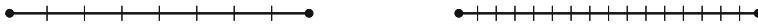
Fig. 1 Two sets of equispaced nodes for a straight open arc. Dots represent fixed nodes, while dashes represent free nodes.
