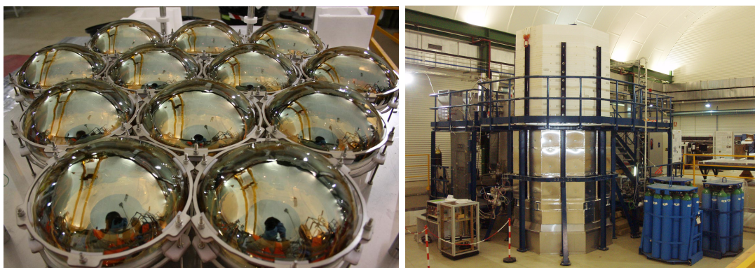
Figure 2.4: Left: The (bottom) PMT array used inside ArDM to detect the scintillation signals S1 and S2. Right: The whole ArDM detector inside the neutron polyethylene shield located at the LSC in Canfranc, Spain. Courtesy of the ArDM collaboration.
