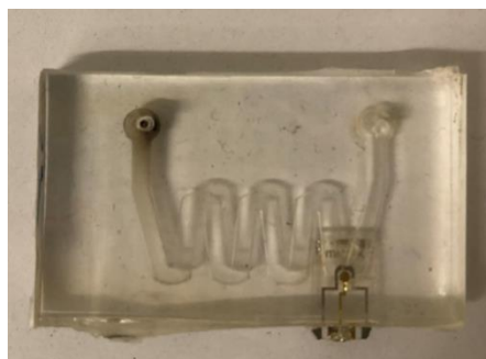
Figure A11 The distribution of PM10 like samples in the microchannel with introducing 0.1 M acetate buffer after 2 min ultrasonic treatment.
