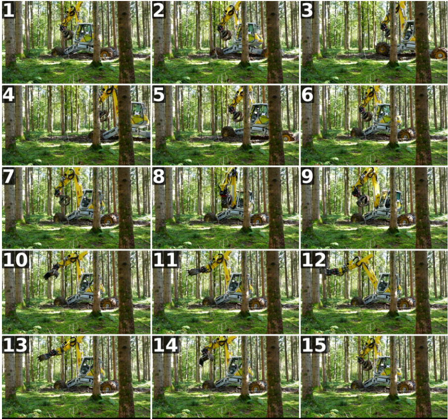
Figure 2.40: Snapshots of an operational cycle between grabbing two trees. HEAP repositioning the base close to the tree (snapshots 1-6) followed by scanning the environment and building a local map (snapshots 7-9). Finally, HEAP grabs the tree by extending the arm (snapshots 10-12) and retracting it (snapshots 13-15). After retracting the arm, the harvester is ready to grab the next tree and whole cycle repeats.
