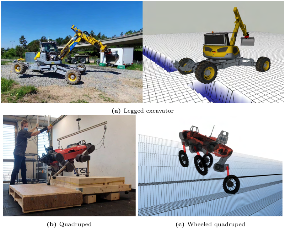
Figure 6.1: a) HEAP overcomes a virtual bridge too narrow to drive over it. Hence, the stepping behavior emerges. We did not dig a ditch in our testing field. However, the map supplied to the planner contains it. Left: HEAP driving on three wheels over the bridge. Right: Visualization of the map the planner sees. b) ANYmal climbing consecutive steps. c) ANYmal on wheels stepping up the stairs (plan visualization). All the motions are also shown in the accompanying video https://youtu.be/4eeqq4Uc192o .
