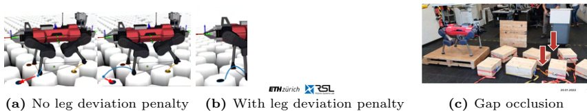
Figure 6.17: a) & b) Improved optimization convergence through penalizing swing leg deviation. We show an example for the LF leg, whose trajectory planned by the MPC is colored in blue. The reference foothold at the end of the swing phase is shown with the blue disk. The initial solution is shown on the left after the optimization iteration on the right. a) Without penalization, the foothold of the optimized trajectory is far away from the reference foothold (distance shown with red arrows). b) The optimized swing motion lands smoothly on the reference foothold with penalization. c) While the LiDAR correctly detects the closer stepping stones, it cannot see holes between the far away stepping stones (marked with red arrows). Hence, the foot placement might be incorrect.
