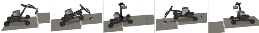
Figure 3.7: Left to Right: HEAP climbing on a 1m block using the stepping gait. The machine exhibits the same behavior as for the gap.
