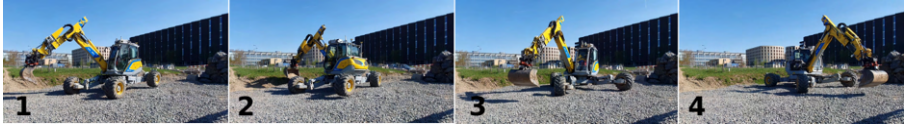
Figure 6.23: HEAP performing a stepping turn in place. The x - y position stays approximately the same, while the azimuth of the chassis changes.
