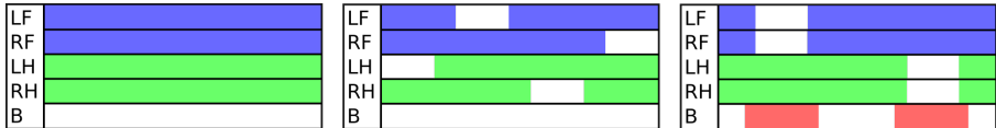
Figure 3.4: Gaits used on HEAP. Color denotes limb that is in contact, and white space denotes that the limb is in the swing phase. All timings are normalized. Left: Driving gait. Middle: Walking without the arm. Right: Walking with legs and the arm.
