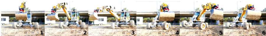
Figure 4.10: Left to Right: HEAP performs a stepping maneuver and reorients its base by 30^\circ . The gait pattern requires it to lift the legs in the following order \{ LH, LF, RH, RF \} . The machine cannot complete the maneuver without using the arm for balancing (e.g., in snapshot 3).
