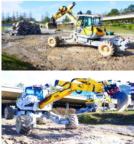
Figure 4.1: Top: A walking excavator has five limbs; an arm, and four legs with a wheel at the end of each leg. They usually operate in muddy and slippery conditions, which requires motion plans with large stability margin. Bottom: Hydraulic Excavator for Autonomous Purpose (HEAP) balancing on three legs while performing a stepping maneuver. A video demonstrating all the motions accompanies this submission.
