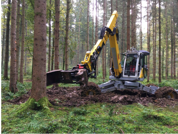
Figure 2.3: Legged excavator navigating to a tree and performing a grab. Human is in the cabin for safety reasons.
