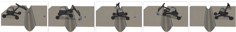
Figure 3.6: Left to Right: HEAP crossing a 3m wide gap using the stepping gait. The coordinate frame marks the goal position. The arm is facing forward initially, but it has to be turned back to step over the gap successfully. This behavior can be seen in the middle figure; HEAP is turning the arm 180 degrees to establish contact on the left side of the gap and thus be able to step to the right side.
