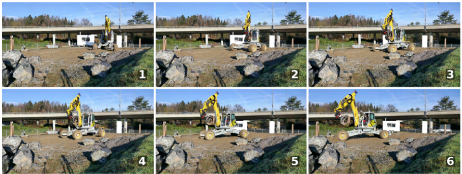
Figure 2.39: HEAP approaching wooden logs at our testing field. We do not show the rest of the maneuver for the sake of brevity. The reader is encouraged to watch the video.
