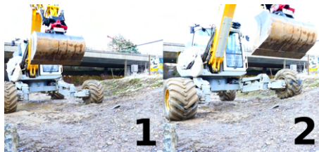
Figure 4.7: Left to Right: HEAP driving forward over a small hill. The front leg adapts its height to the ground height, despite motion planner producing plans under the flat ground assumption.
