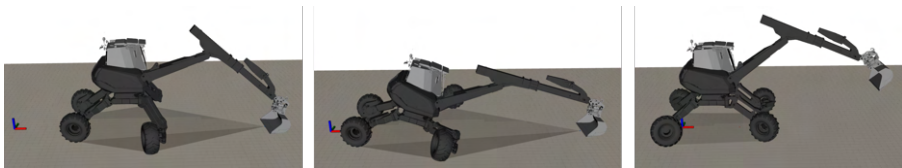
Figure 3.9: Left to Right: HEAP moving from (x, y) = (5, 0) m to (x, y) = (0, 0) m while simultaneously optimizing over the gait timings. Left: The base has to move where the coordinate system axis are. Middle: Even with the fully extended arm and tilted base, it is still too far from the goal position to reach it without changing the gait timings. Right: The contact timings change and the contact is broken.
