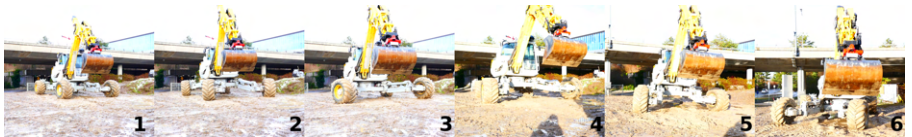
Figure 4.9: Left to Right: HEAP performs a driving maneuver. The base is commanded to move forward and left (frames 1-3). Subsequently, we command the machine to drive back to the starting point (frames 4-6). The planning and control pipeline naturally discovers the crab steering mode of the machine.
