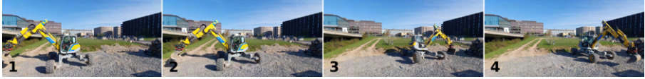
Figure 6.24: HEAP performing a stepping turn and moving laterally. The chassis keeps the azimuth approximately the same as at the beginning of the maneuver.
