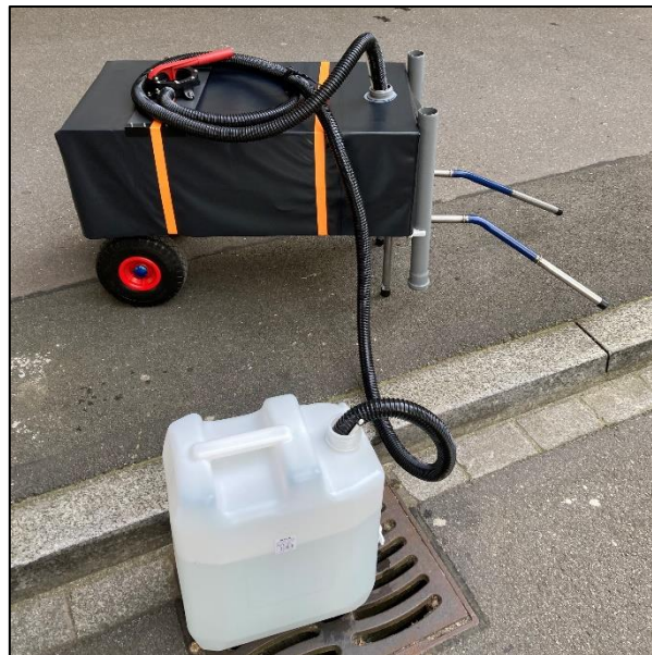
Figure 17: Urine collection trolley during the pumping process.
