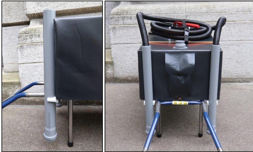
Figure 13: Side and front view of the pipes used for storing the hose ends.
