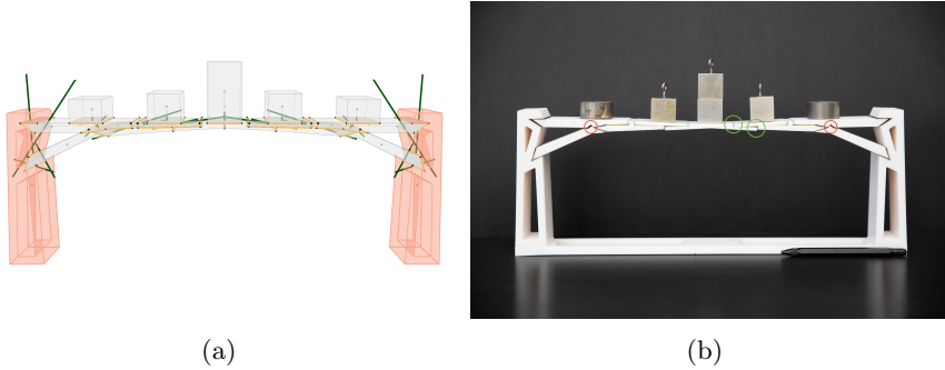
Figure 7.4: (a) Bridge in its final configuration and subjected to additional loads. (b) The span of the 3D printed model is 40 cm, the net mass of the bridge (excluding the supports) is 319g, while the mass of the externally applied loads is 1208g. The red circles denote two sharp wedges designed to guarantee that the two external elements are in the right position.
