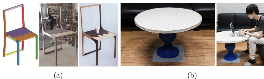
Figure 2.3: Embedding structural equilibrium analysis of complex assembly in the design tool enables various applications, including furniture design: (a) analysed and fabricated chair joinery design from Yao et al. [2017]; and, (b) the LEGO table was structurally designed and fabricated by Luo et al. [2015].
