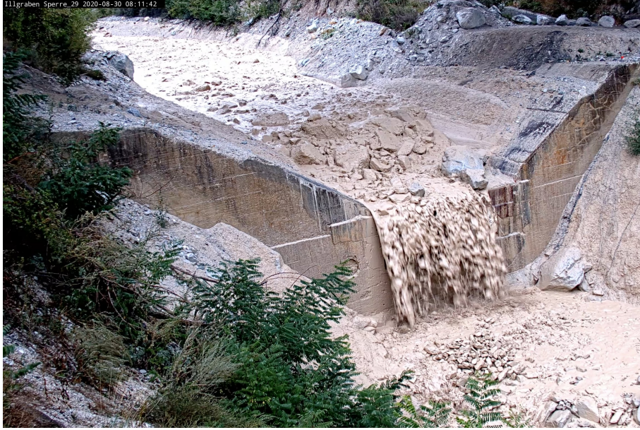
Figure 3.1: A debris front passes a concrete check dam at the Illgraben test site on August 20, 2020. Note the blocky front and watery tail. The front appears to dam the muddy fluid flowing behind; the rocks in the tail appearing completely submerged in the muddy fluid. Saturation increases from front to tail. Photograph WSL.
