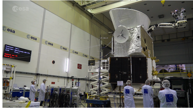
Figure 1.1: The BepiColombo spacecraft stack undergoing vibration tests at the European Space Agency. Credit: ESA - European Space Agency, CC BY-SA 3.0 IGO.
