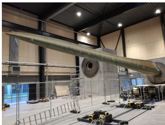
Figure 1.3: A 14.3 m long research WT blade manufactured by Olsen Wings and tested by DTU Wind Energy at the DTU Large Scale Facility. Credit: DTU Wind Energy.
