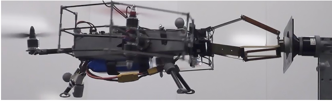
Fig. 7: APhI experiment with the AM pushing on a surface connected to a F/T sensor.
