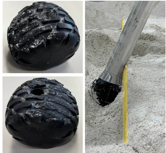
(a) ANYmal feet heavily damaged by slippage after a few minutes walking on the slopes. (b) Robot stumbles at the boundary between sand and stone slabs highlighted in yellow.
