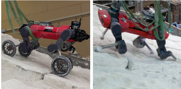
(a) The hybrid wheeled-legged version of ANYmal, with its wheels slipping. (b) The standard legged ANYmal critically slipping and involuntarily contacting the ground with the knees.
