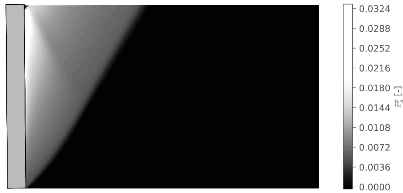
Fig. 53: Cumulative deviatoric plastic strain for \varphi = 30^\circ and \delta = 20^\circ .
