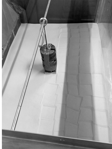
Fig. 78: Compaction of the backfill by applying a static load.
