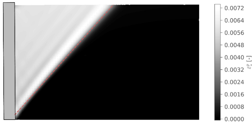
Fig. 48: Cumulative deviatoric plastic strain for \varphi = 30^\circ and \psi = 5^\circ using a coarse mesh (element size = 0.1 m).
