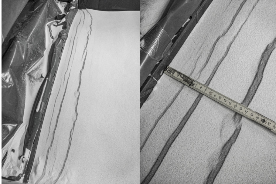
Fig. 86: Shear bands observed from the top after the conclusion of test C2D.
