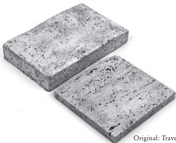
Original: travertine Imitation: sponge und plaster
