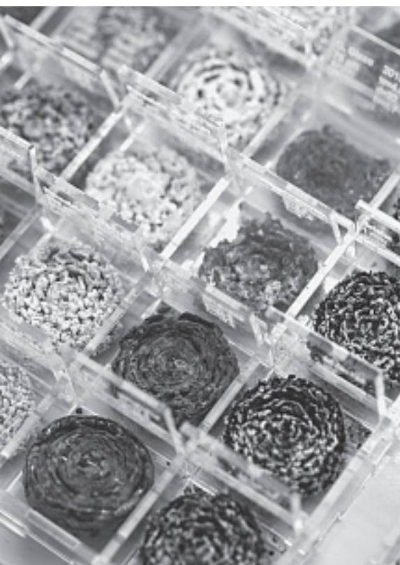
Grown building elements from building rubble and bacteria Photo: Kilian J. Kessler
