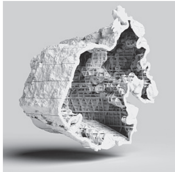
3D sand-printed parametric freeform formwork system for freeform constructions
