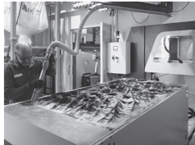
Desanding of a 3D-printed ceiling prototype at Christen Guss AG
