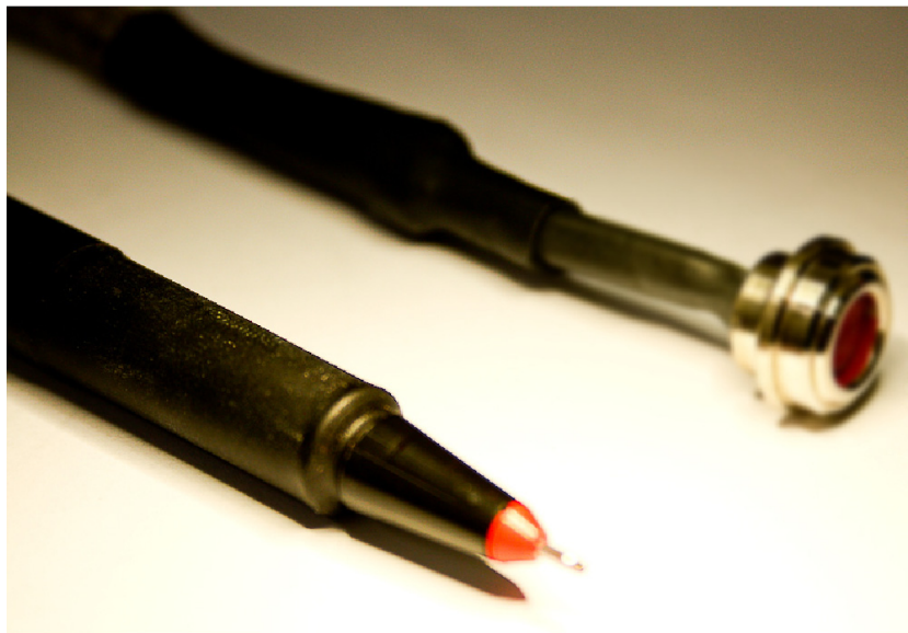
Fig. 38. High temperature fast response probe presented with a pen for scale comparison. The presented probe replaces the nozzle at the dispenser outlet.
