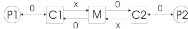
Figure 42: Memory model for the file system. Two processes P1 and P2 communicate through the file system modeled by two local memories C1 and C2 and a global memory M . On some paths it takes zero time for the data to propagate from one element to the next. On others it takes a time x which is a positive bounded random variable.
