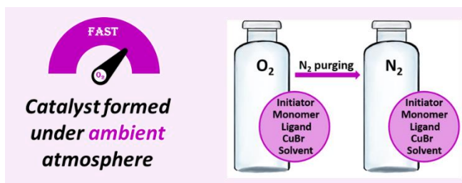
Scheme 2. 3: Schematic representation of oxygen-enhanced ATRP in which the formation of the catalyst occurs under ambient atmosphere.
