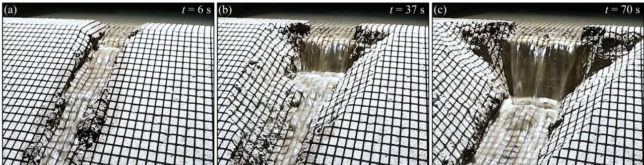
Figure 4. Progressive surface erosion of shell material leading to (a) initial breach channel, (b) incision of breach channel and core exposure, and (c) further incision of breach channel with unstable side slopes.
