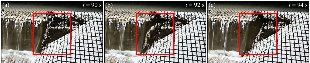
Figure 6. Filter erosion: (a) before, (b) during, and (c) after a mass detachment of apparent-cohesive material.
