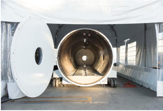
Figure 7—Vacuum Chamber used for testing
