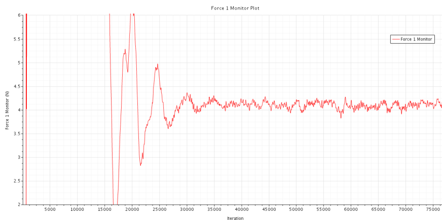
Figure 6.58: Force Monitor Plot of Version B at 0.01 bar
