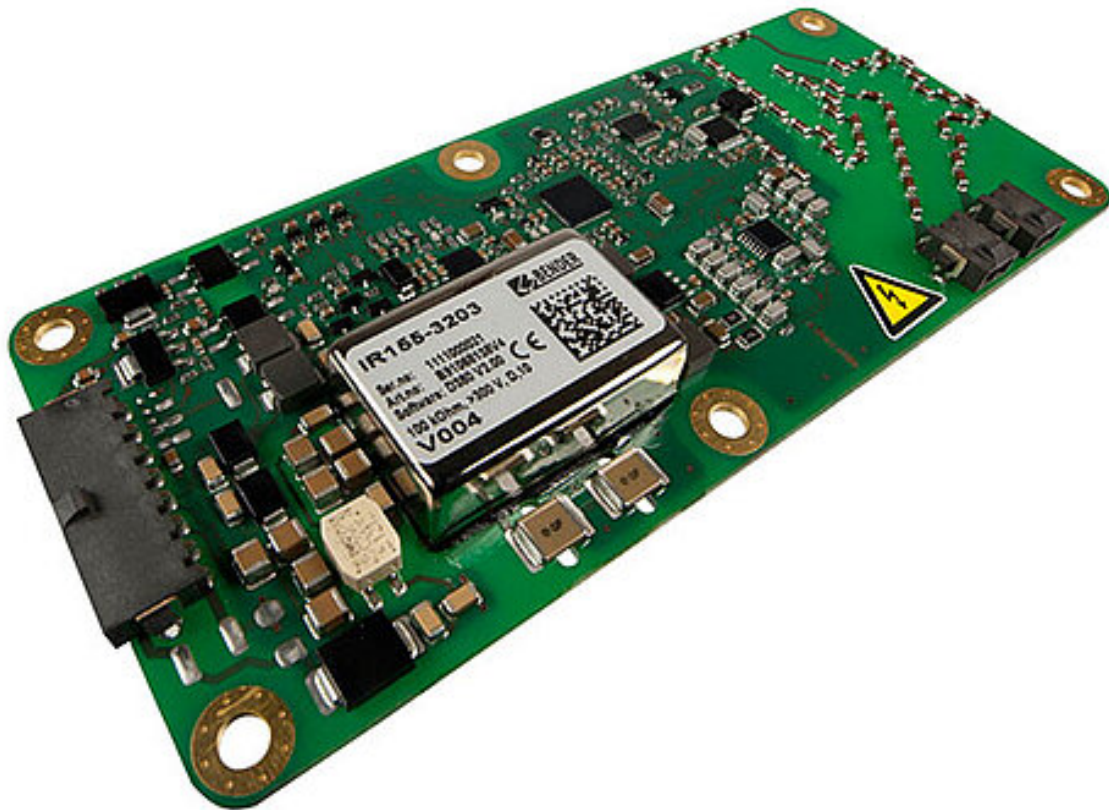
Figure 4.21: Isolation Monitoring Device (IMD) used in the Prototype [19]
