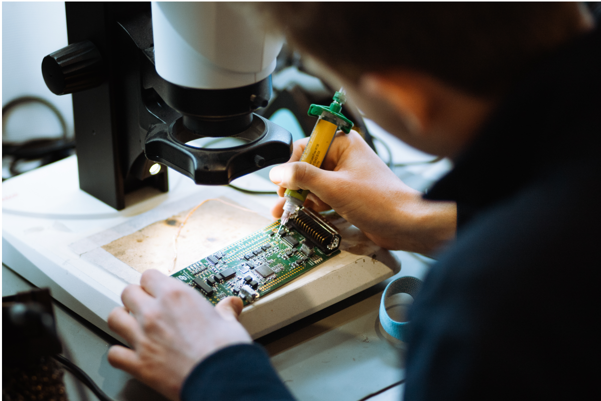
Figure 4.5: The Master Board being soldered
