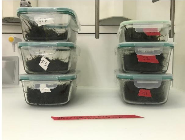
Figure S-7.2. Ammonia pretreatment conducted in glass containers with a lid to avoid ammonia loss. To identify the dose and treatment time, pretreatments were conducted in triplicate.
