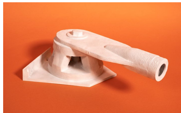
Figure 3. Test print in scale 1:1 of the mesh model
