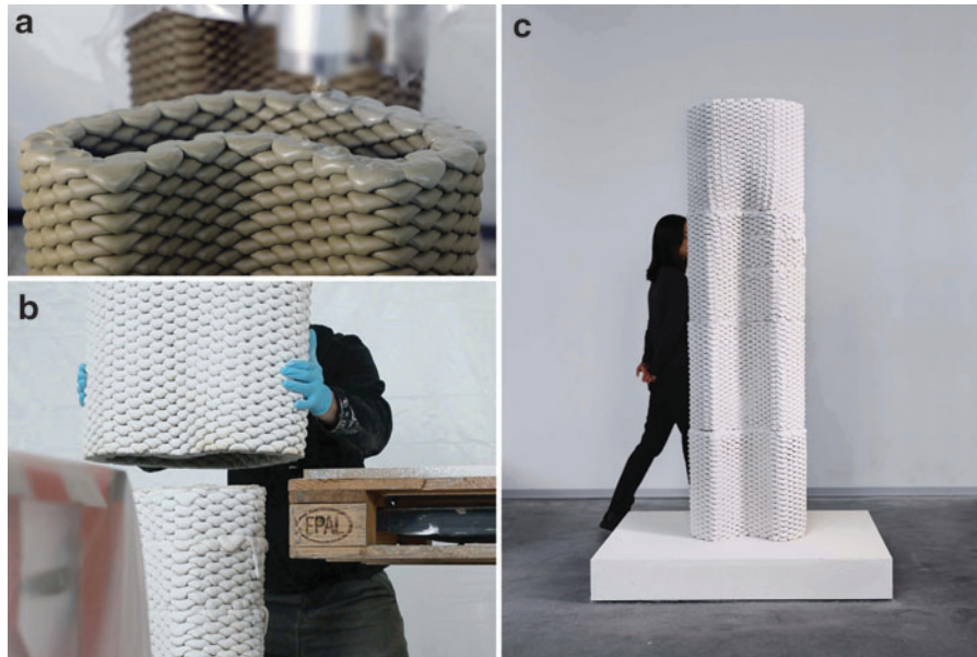
FIG. 8. The final prototype showing (a) 3D-printing process, (b) manual assembly, and (c) the finished structure.
