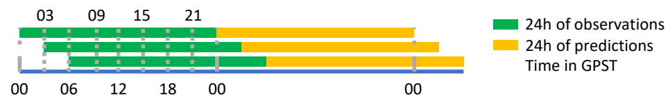
Figure 1. The schematic diagram of the GFZ 3-hourly ultra-rapid orbit products.
