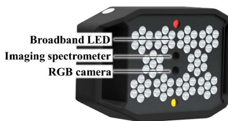
Figure 1. Hyperspectral imaging system, HAIP BlackMobile
