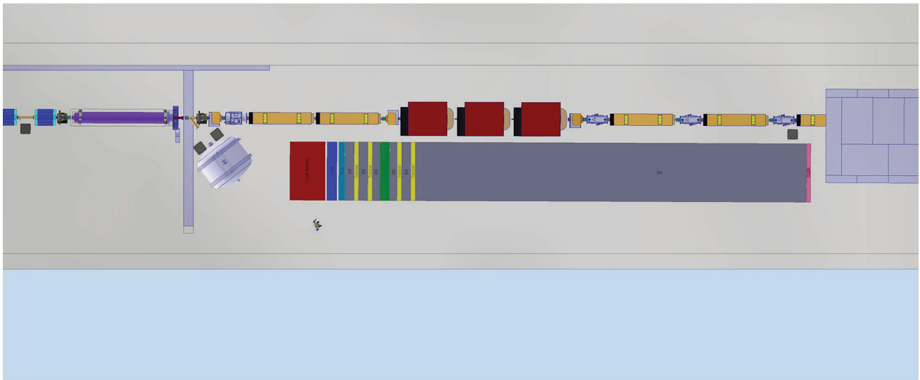
Fig. 93 Top view of the SHADOWS detector in the experimental hall. The beam is entering from right to left. The shielded area containing the TAXes dump is visible at right. SHADOWS detector is sketched at the bottom of the figure. The dimensions of the detector and the beamline elements are to scale
