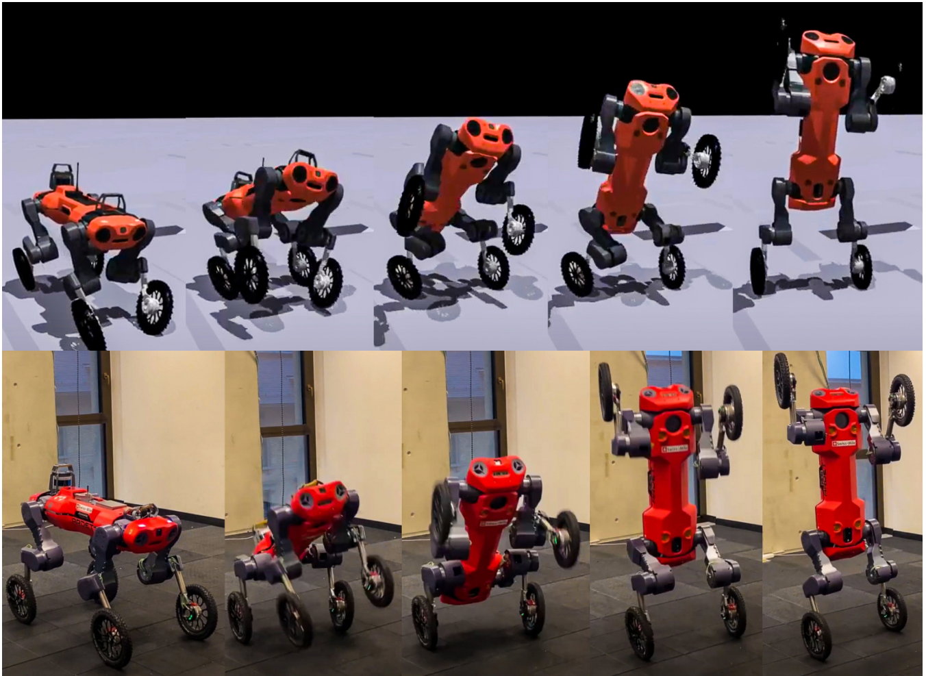
Fig. 4. Stand up-sequence in simulation and on the real robot. The policy is able to stand up, navigate large distances on two legs, and finally sit down again using the stand-up motion prior.
