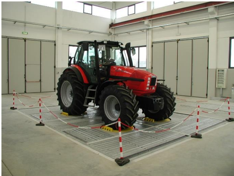
Figure 10. Layout of the “four poster” at the CREA-IT research centre.
