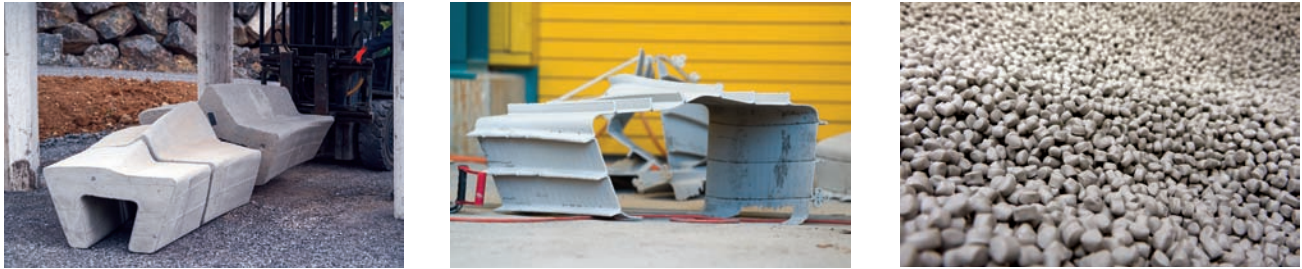
△ Figure 5. Case Study B. (a) Eggshell benches, (b) removed formwork, (c) recycled rPIPG regranulate.
