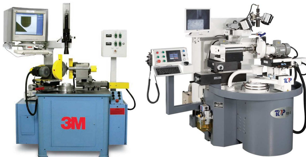
Figure 2.10 – Dressing machines for conditioning metal bonded grinding wheels: 3M™ type E339V (left) [3M2011] and Atrump type TD1 (right) [ATRU12]
