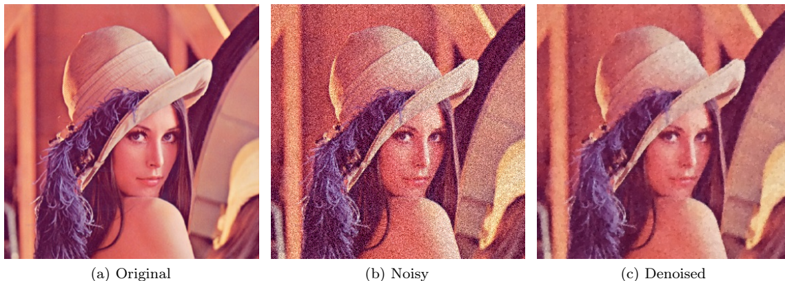
Figure 4.2: Denoising of a color image using the linear vectorial color model which corresponds to the manifold \mathbb{R}^3 (a) Original image "Lena.jpg", 361 \times 361 px, 8 bit color depth (b) Component-wise Gaussian noise \mu = 0 , \sigma = 0.1 added (c) Denoised, IRLS with \lambda = 0.1 , 5 IRLS steps, 1 Newton step per IRLS step
