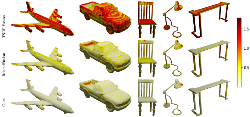
Figure 5.6: Mesh Accuracy (M.A.) visualization on ShapeNet meshes. Our method consistently reconstructs more accurate meshes than the baseline depth fusion methods. Especially thin geometries (table/chair legs, lamp cable) are reconstructed with better accuracy.
