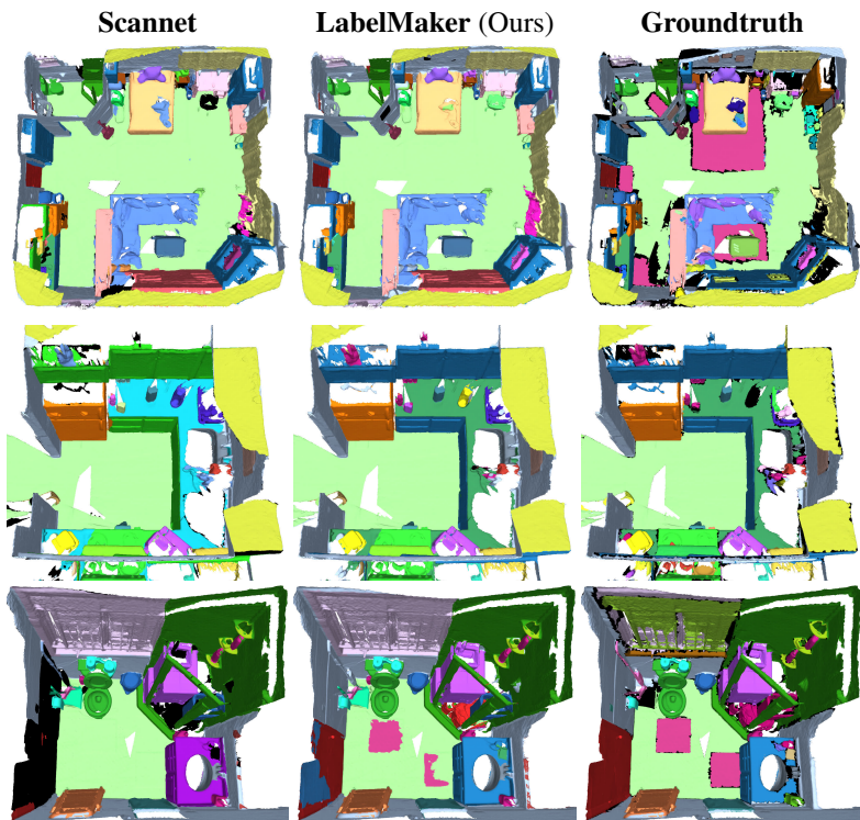
Figure 9.5: Dense 3D labels for ScanNetv2 [Dai et al., 2017a]. We generate more consistent labels compared to human annotators and preserve rare classes (e.g. swivel chair in front of the desk). Further, the labels are more complete (e.g. wall in bathroom) and we can capture all object in the scene (e.g. dustpan in bathroom).
