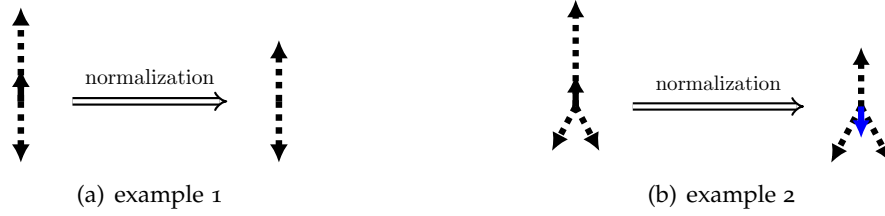
FIGURE 6.3: The expected update of NSGD can vanish (example 1) or be in the opposite direction (example 2) of the true gradient. The solid black arrow represents the true gradient and the dashed arrows are the possible stochastic gradients (with equal possibilities). The solid blue arrow is the expected direction of NSGD update.
