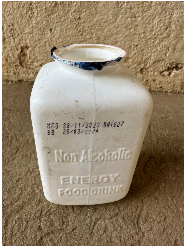
Figure 23: Empty Super Maheu bottle. Some aluminium foil and parts of the tie layer remained on the bottle rim.
