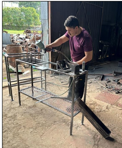
Figure 20: Different stages of manufacturing of the second prototype. a) Sealed components of the water module, b) Reinforcements being welded to the workbench, c) Spray painting of the workbench
