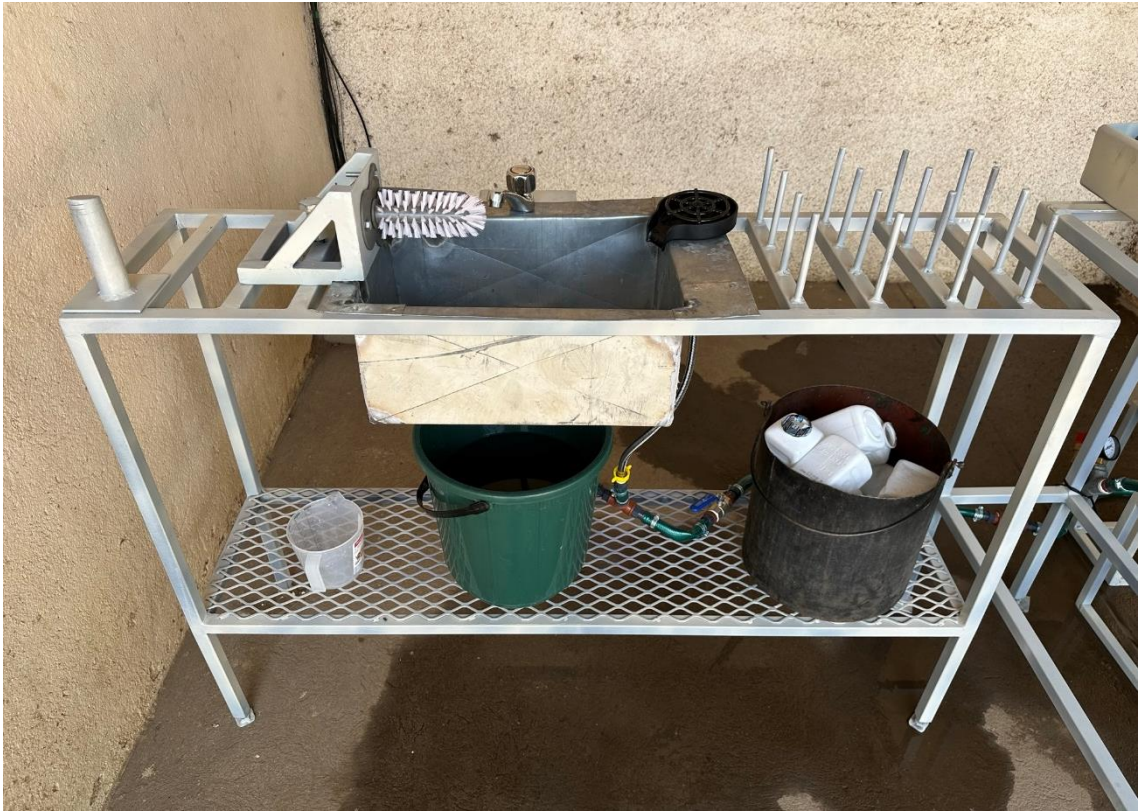
Figure 22: Front view of the inflation and cleaning module as installed in the second prototype. The inflation module is located on the left, the storage pins on the right. The cleaning module in the middle includes: Brush, Sink, Tap, Rinser.
