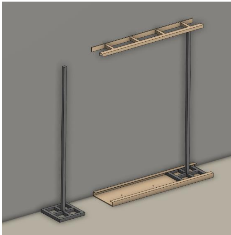
Figure 13: 3D-representation of the loading process. Bottles are stacked on the pole and slide into the rail
