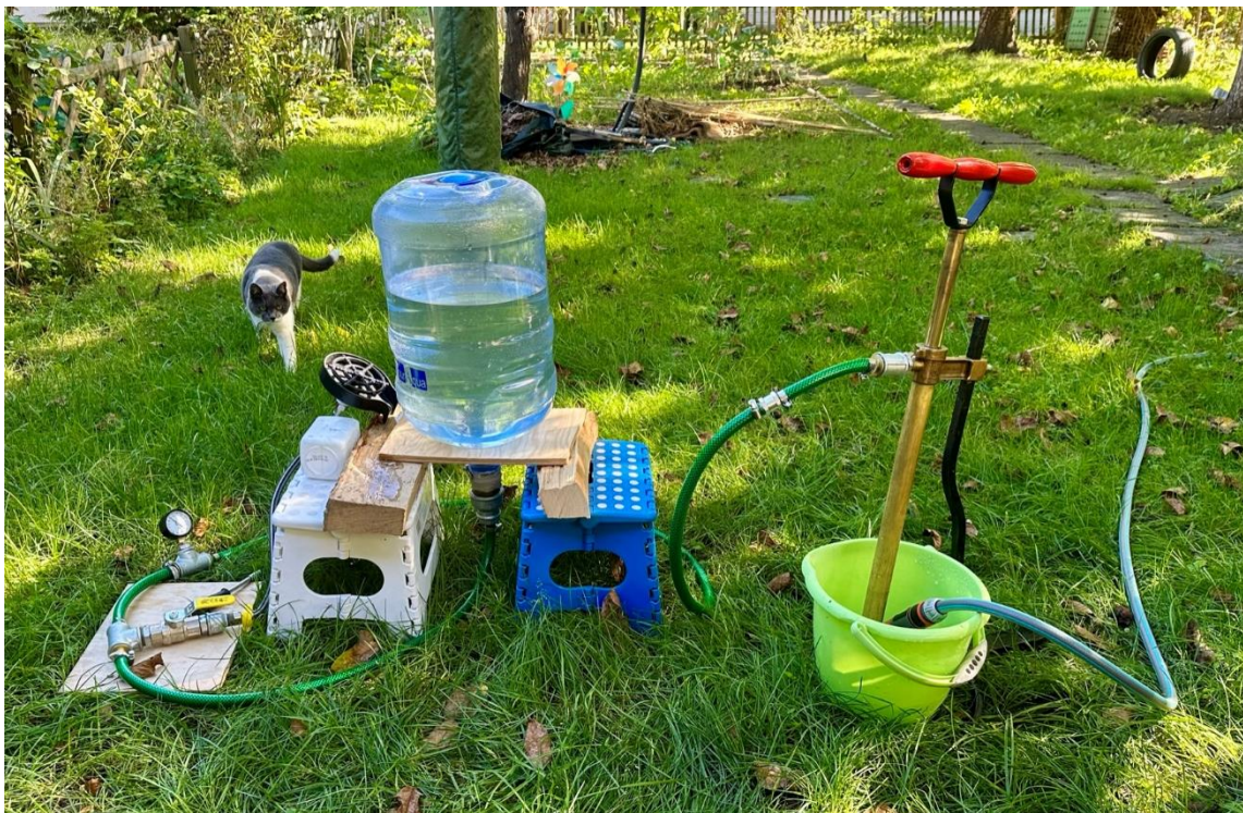
Figure 17: First water module prototype. The glass rinser is connected as primary water outlet.
