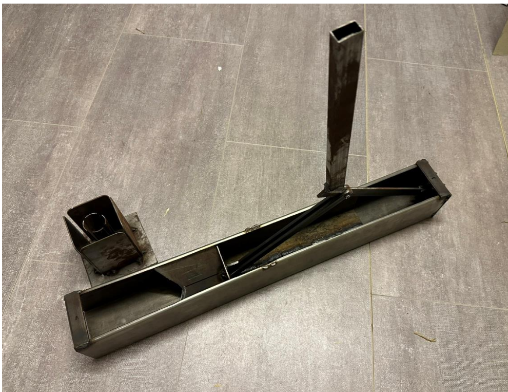
Figure 18: First prototype of the cutting module. The bottle adapter is removed from the guide rail.
