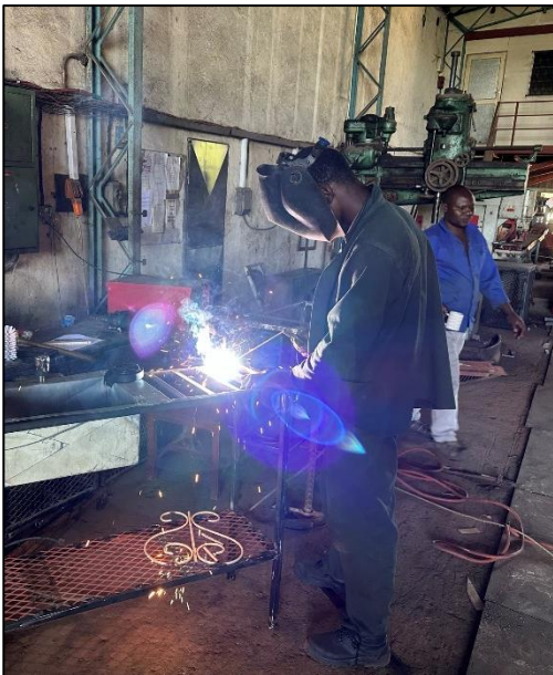
Figure 20: Different stages of manufacturing of the second prototype. a) Sealed components of the water module, b) Reinforcements being welded to the workbench, c) Spray painting of the workbench
