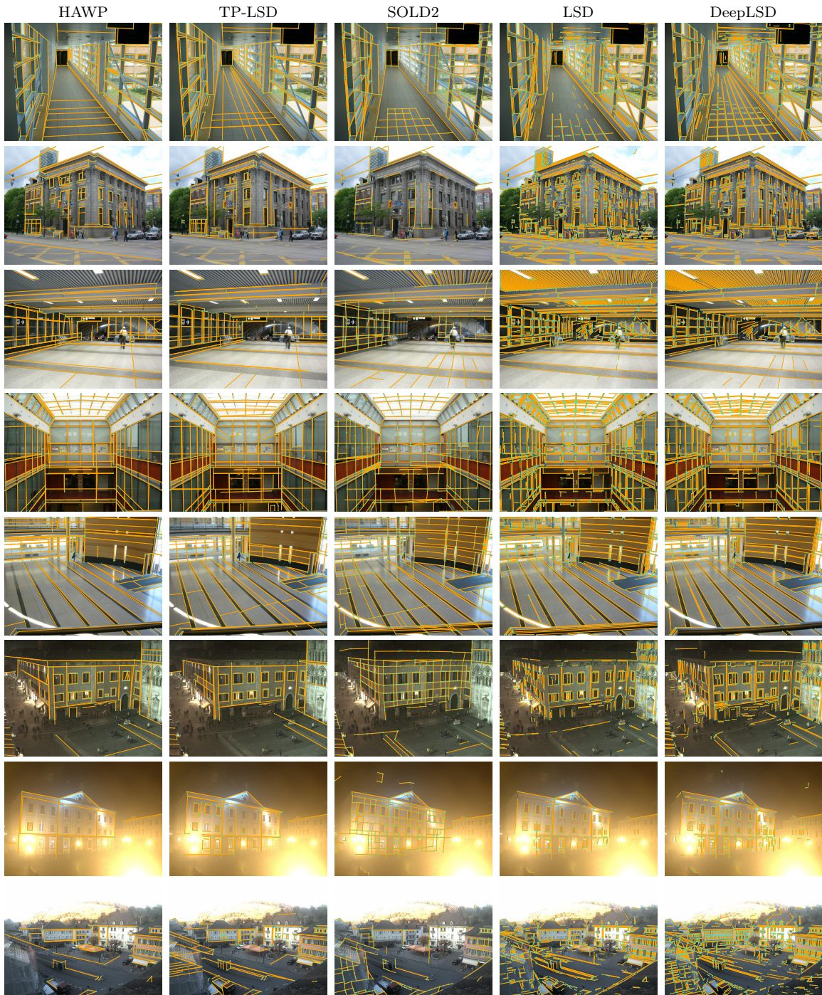
Figure 4.12: Visual comparison of line detectors. First five rows: the lines of DeepLSD (here, without line refinement) are more complete and accurate in urban scenarios (images from the YorkUrbanDB dataset [Denis et al., 2008]). Last three rows: when employed in challenging scenarios such as by night, over-exposition and low image quality, DeepLSD can detect more relevant lines than the other baselines (images from the Day-Night Image Matching (DNIM) dataset [Zhou et al., 2016]).
