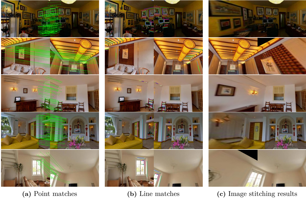
Figure 5.7: Examples of GlueStick matches on image pairs of SUN360 [Xiao et al., 2012]. We provide the point and line matches, as well as the stitching of the two images using the resulting matches.
