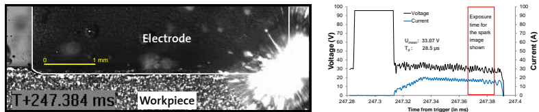
Figure 3: Time synchronised visual and electrical information of the EDM spark.
