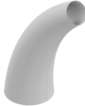
(b) 3D model of a printed sample 2 with R=314 mm, \varnothing_1=100 mm and \varnothing_2=50 mm.
