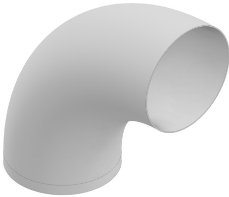
(a) 3D model of a printed sample 1 with R=150 mm and \varnothing=100 mm.
