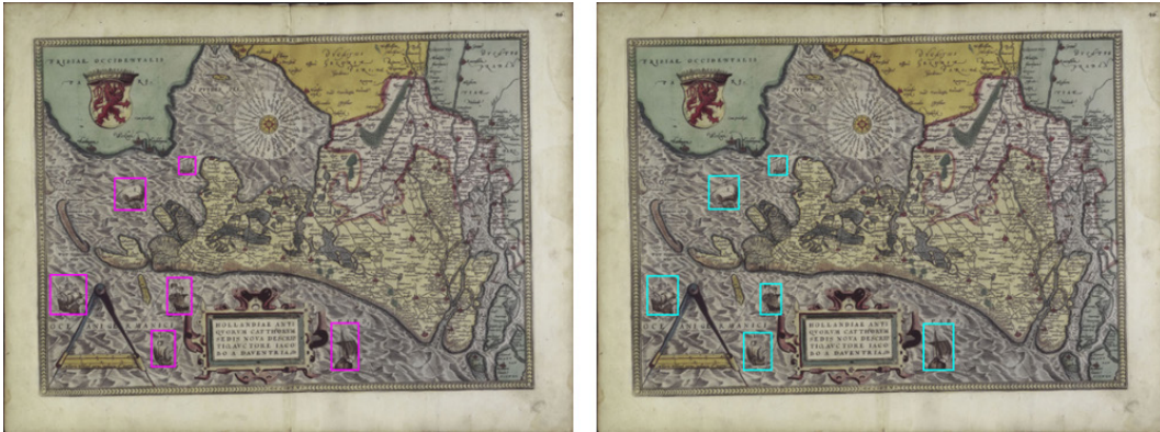
Figure 3.7: Ground truth (left) and detected bounding boxes (right) with the best trained Faster R-CNN model (AP: 32.8%) for large, freestanding ships (original image source: Sammlung Ryhiner 22 )
