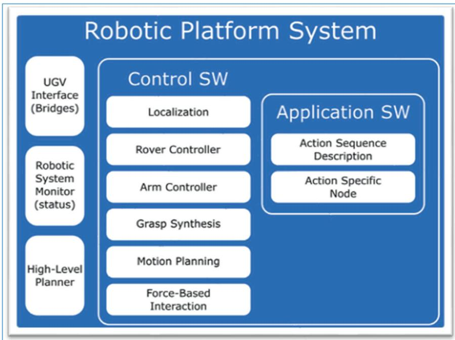
Figure 11.11. Overview of the robotic platform components.
