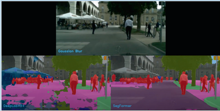
Figure 11.8. An example of segmentation robustness on a corrupted (gaussian blur) sample from Cityscapes-C benchmark dataset. It is compared to a previously state-of-the-art model, DeepLabV3+. Source [1].
