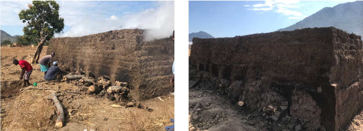
Figure 1.6: Burning of the stacked bricks using fuelwood.
