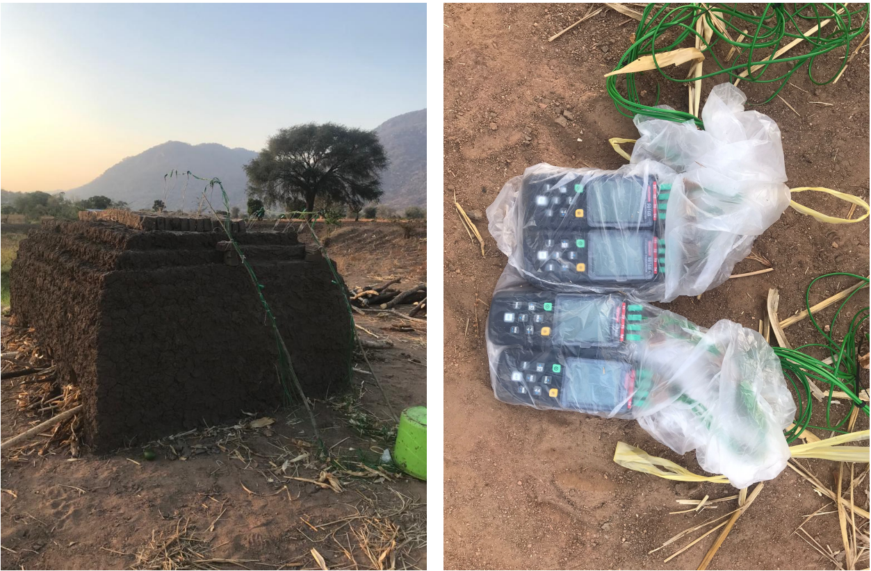
Figure 2.6: Cabling and data loggers during the firing process.
