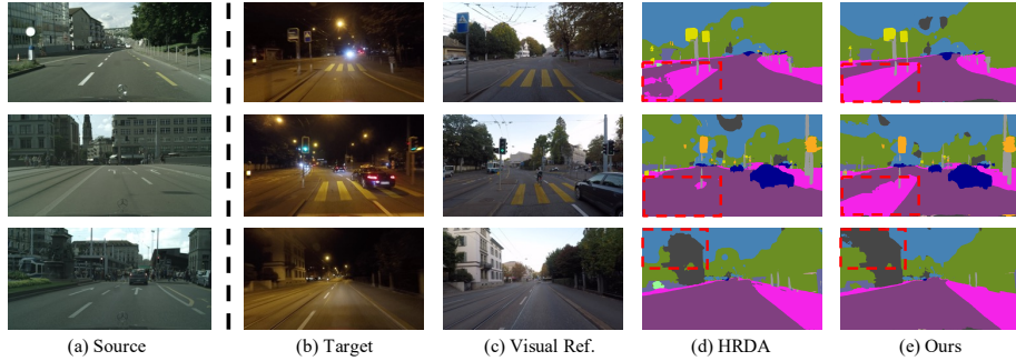
Figure 5.4: Qualitative Comparisons for UDA Semantic Segmentation , under Cityscapes \rightarrow Dark Zurich. (a) shows the example of Cityscapes images. (b) includes the Dark Zurich images. (c) covers the day images corresponding to the night images in (b) for better visual references. Note that, the day images in (c) are only used for visualization references, but are not used for training and testing. (d) and (e) are the segmentation results for (b) from HRDA [76] and our method, respectively.
