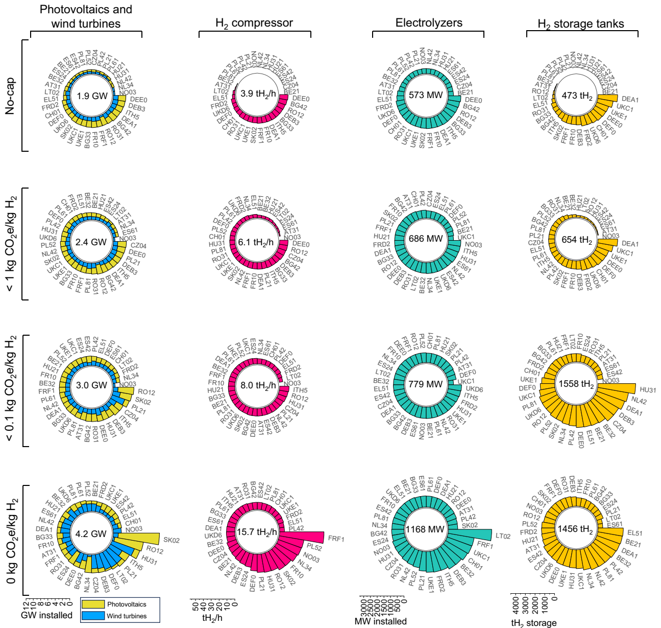
Fig. 3 | Optimal electrolytic hydrogen production system (EHPS) design across Europe. Regions coded according to the NUTS-2 level of the Nomenclature of Territorial Units for Statistics (NUTS) system (Supplementary Table 1) and ordered by installed capacity. Values inside the spirals refer to the mean installed capacity of the respective component in European plants given emission constraints (caps) on the lifespan well-to-gate carbon dioxide equivalent (CO 2 e) content of
